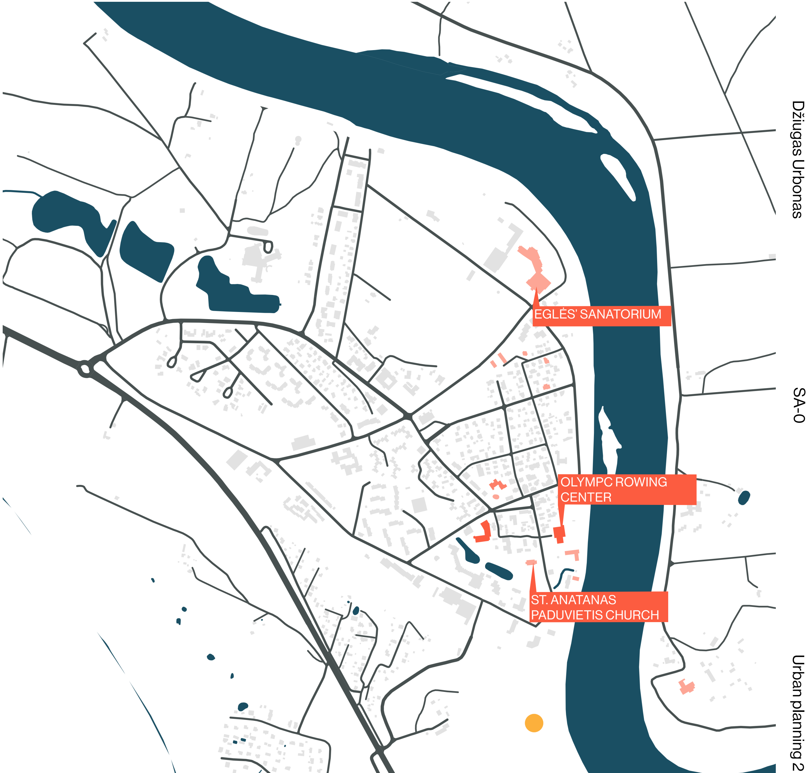
Map of buildings visible from Vytauto Kalnas. Made using viewshed methodology from a point cloud DSM
