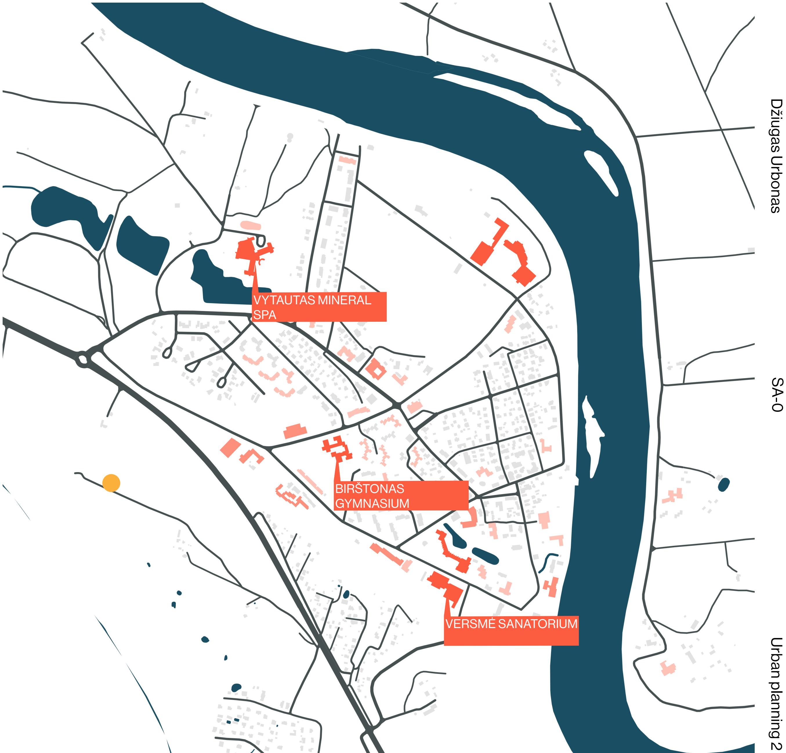
Map of buildings visible from the observation tower. Made using viewshed methodology from a point cloud
