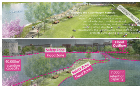
Cloudburst system, Copenhagen
